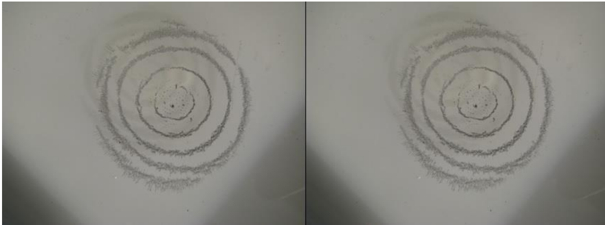
Fig.4. The original pictures of symmetrical ring structures. Conditions: d=38 mm; h=33 mm (left) and d=38 ; h=34 mm (right)
